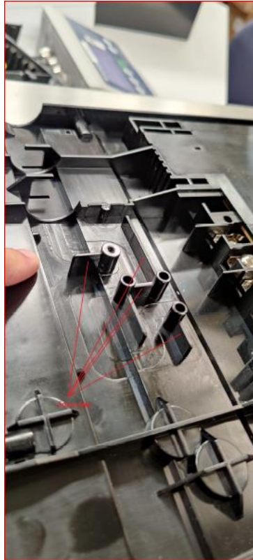
Fig. 2.: The bosses and ribs cord guiding elements configuration
