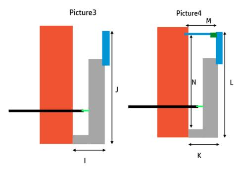
Picture3 describes the antenna distance I+J represent the PIFA type "quarter wavelength" when there is no signal from the fingerprint sensor
