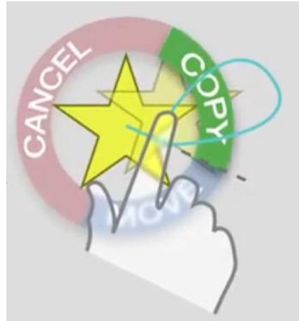
Fig. 4: The target can be closer to the source than the radius of the ring menu
