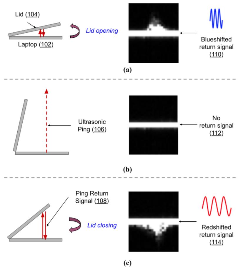
**Fig. 1: Detecting the state of a laptop lid using an ultrasonic ping signal**
