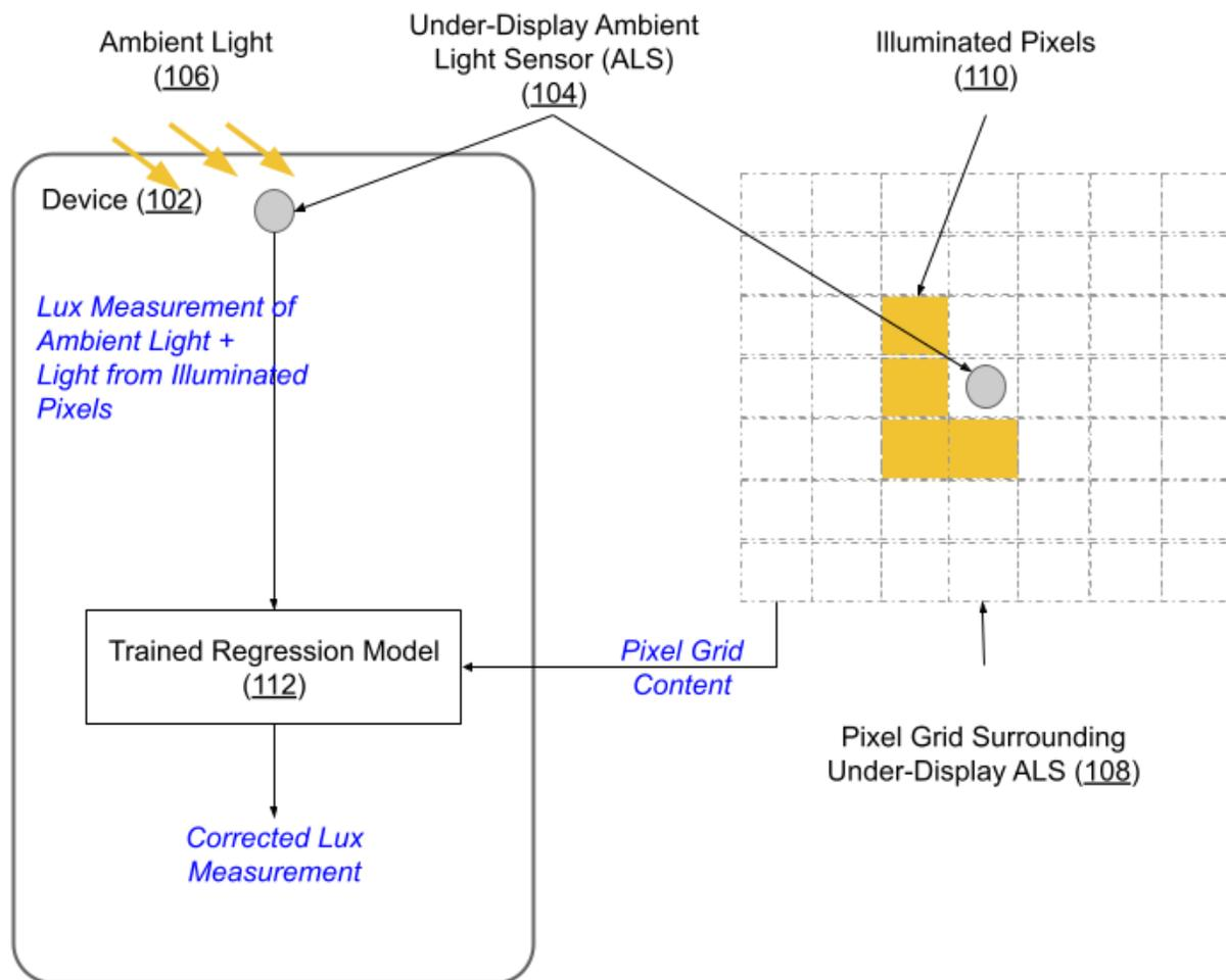
**Fig. 1: Subtracting the impact of illuminated pixels that surround an under-display ambient light sensor**
