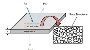
Figure 4: In-and-out coming power of EM wave through metal foam
