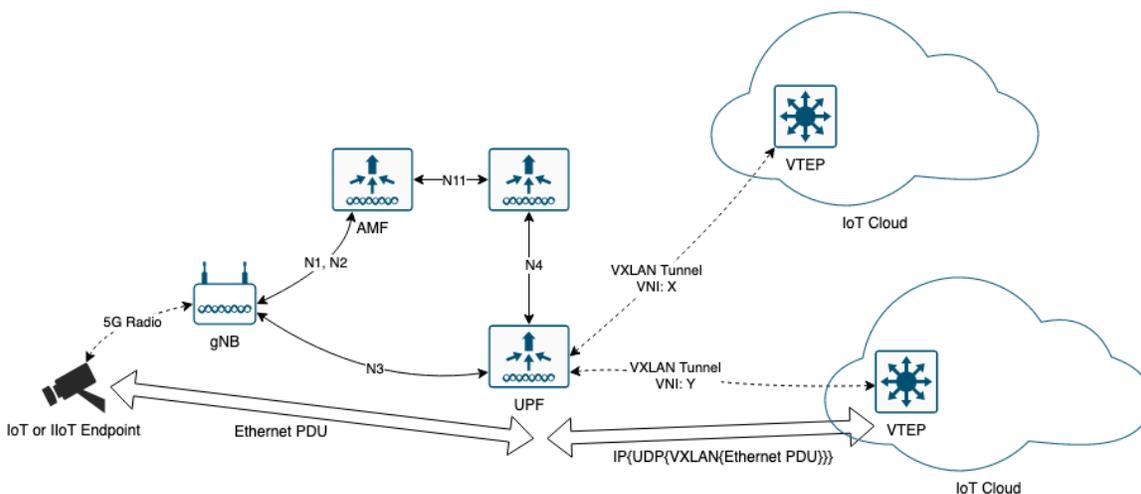
Figure 1: Example 5G Network Architecture
