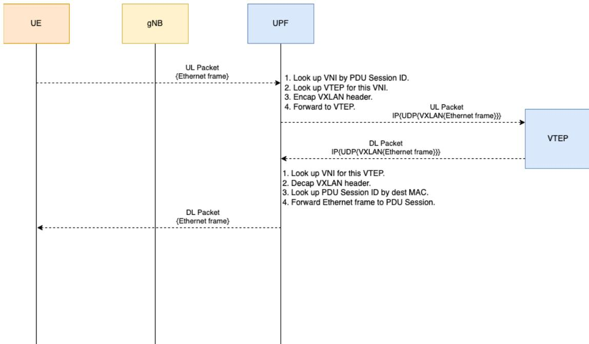
Figure 3: Example UPF UL/DL Frame Processing Call Flow
