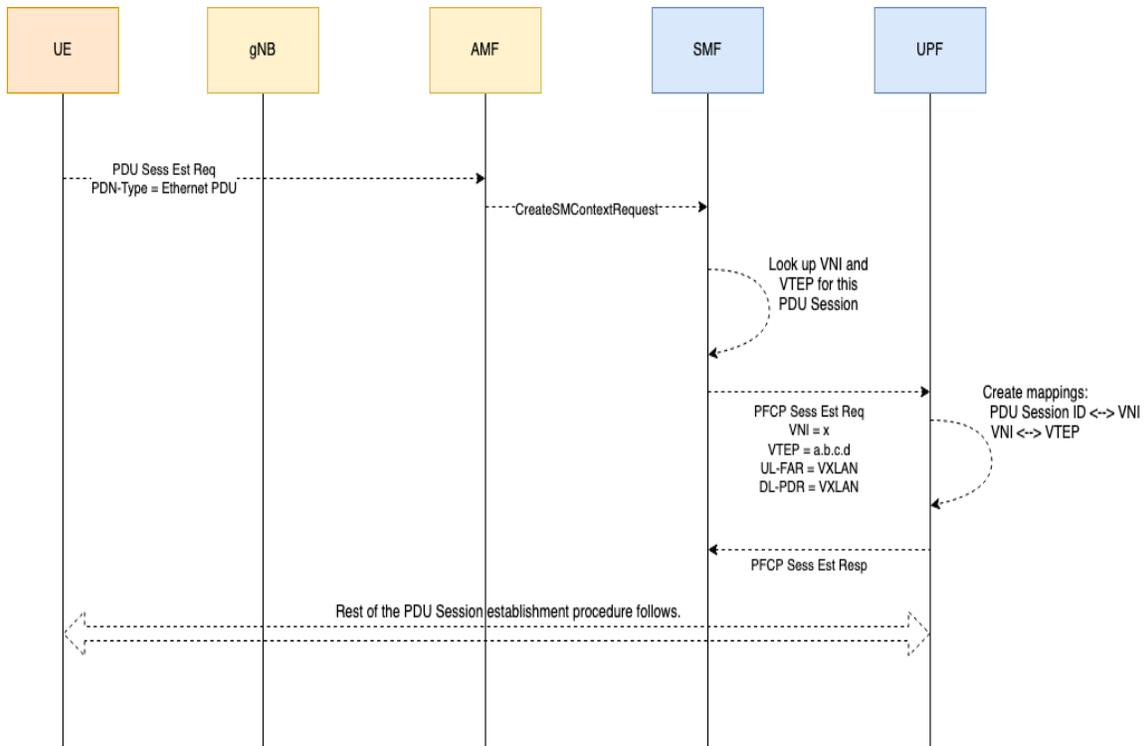
Figure 2: Example Control Plane Call Flow
