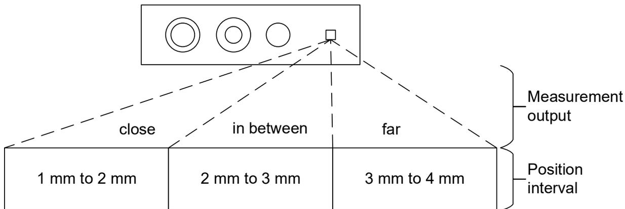
**Figure 2. Focusing element(s) position intervals based on laser proximity sensor measurement output.**
