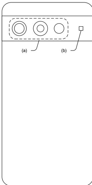
**Figure 1. Smartphone having a camera module (a) and a laser proximity sensor (b).**
