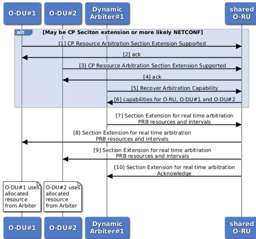
Figure 1: Exemplary Call Flow Illustrating O-RU, O-DU, and Arbiter Communications
