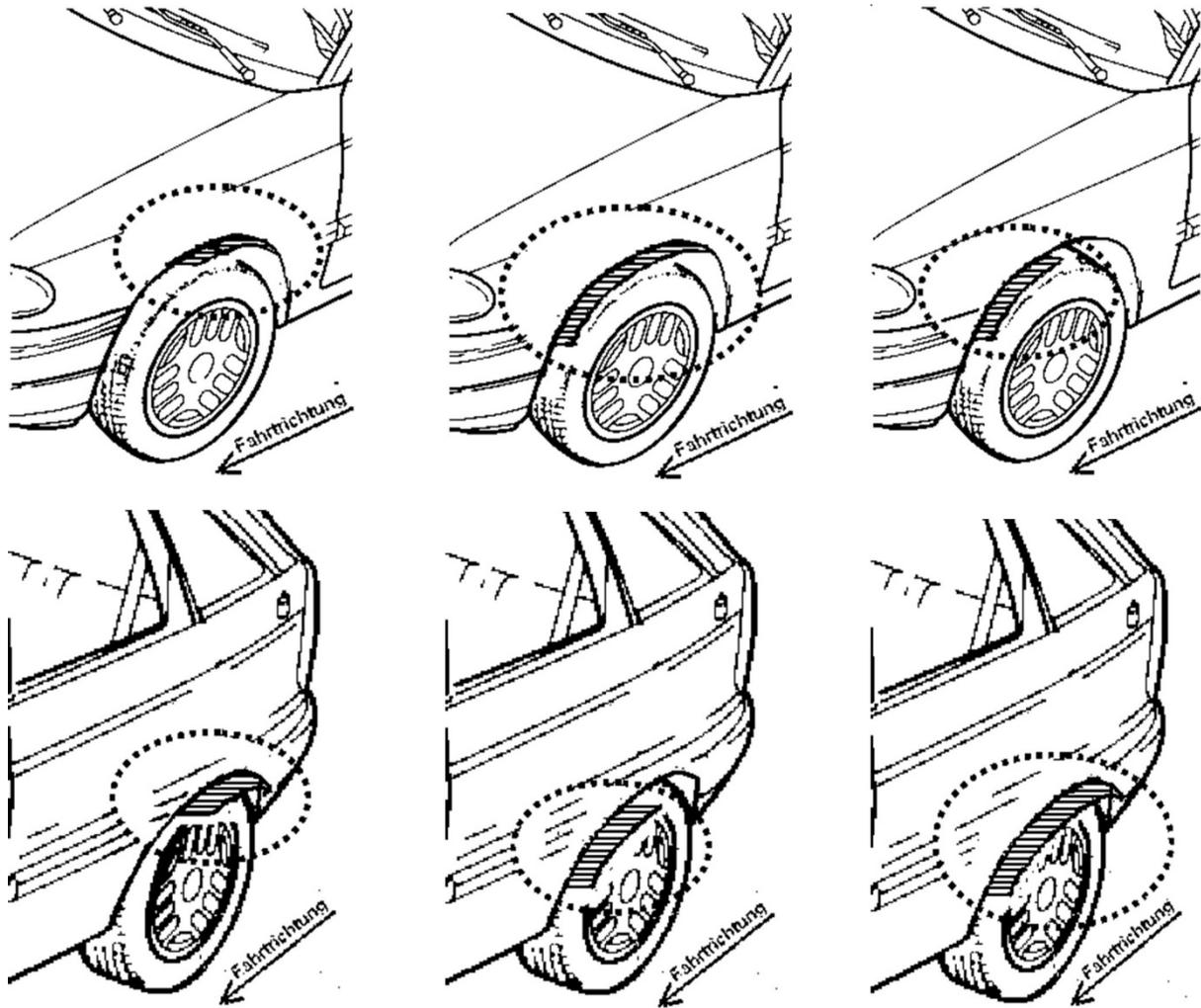
**Fig. 2 shows the wheel tread prescribed by the KBA on the front axle (30 grd. front - left picture - 50 grd. rear - right picture - and shown complete on the front axle in the centre picture and the wheel tread prescribed by the KBA on the rear axle (30 grd. front - left picture - 50 grd. rear - right picture - and shown complete on the rear axle in the centre picture).**
