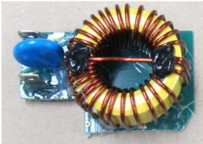
Figure 4 shows different ferrite inductors and different placement of the capacitor (shown as blue component)
