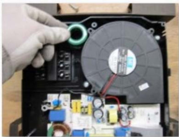
Figure 2 shows area at the entry of power supply line dedicated for the variable EMC filter board.
