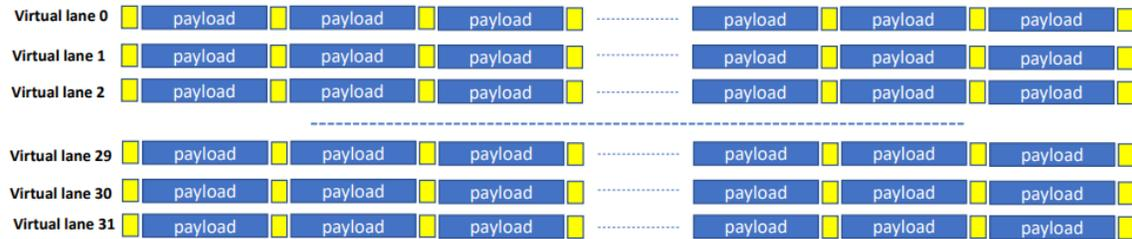
*Figure 6: Exemplary Reassembled 800GE Stream*
