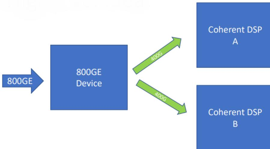
*Figure 1: Illustrative Splitting of an 800GE Stream*
