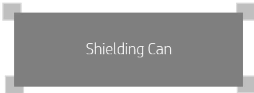
Figure 3. Shielding Can with conductive sponge at 4 corners
