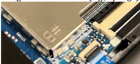
Figure 5. Typical shielding can corner is not sealed very solid if only using metal sheet
