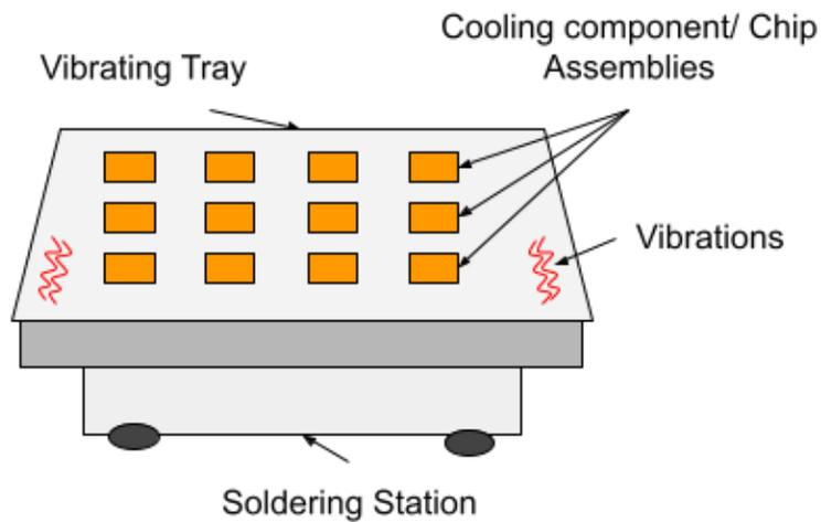
**Fig. 2: Mechanical vibration can be applied during direct soldering**
