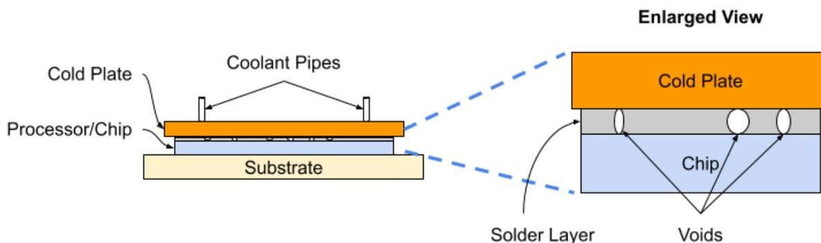
**Fig. 1: Heat transfer can be hindered by voids formed during soldering process**
