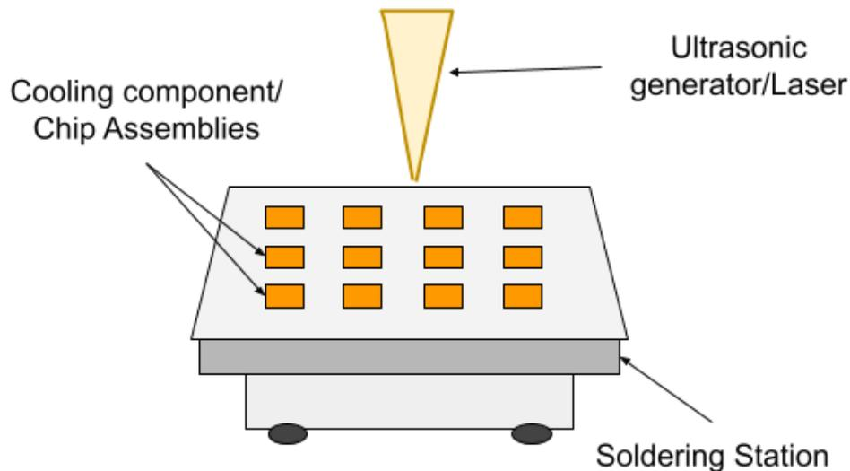
**Fig. 3: Non-contact vibration applied during direct soldering**
