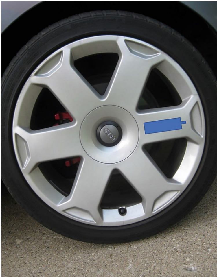
Figure 1: Exemplary positions of the pressure reservoir (blue) integrated into the rim.
