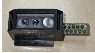
Figure 3 – Spectrophotometer sensor to detect media width
