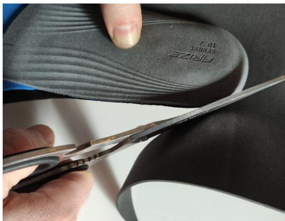
*Figure 1: Top cover manual cutting*
