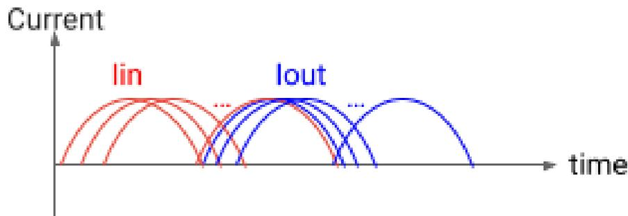
**Fig. 3: A battery of elementary SC-VR cells delivers a nearly constant output current ( $I_{out}$ )**
