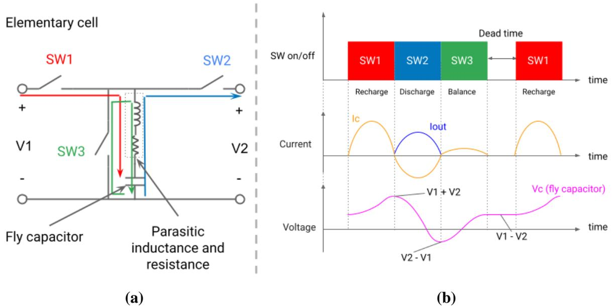
**Fig. 1: Integrated, switched-capacitor voltage regulator with DTC: (a) topology; (b) operation**
