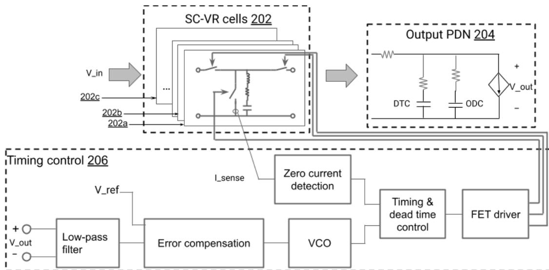
**Fig. 2: Developing a greater power output by arranging VR cells in parallel and by sequencing their operations**
