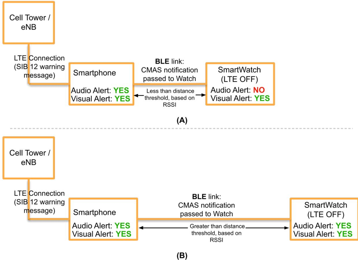
**Figure 1: (A) The smartphone and smartwatch are in close proximity, as detected by RSSI, such that only one device (the smartphone) sounds an alert; (B) The smartphone and smartwatch are relatively far apart, as detected by RSSI, such that only both devices sound the alert.**
