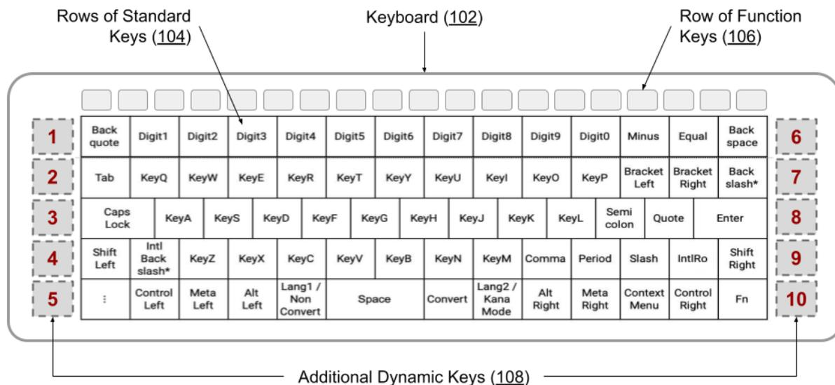
**Fig. 1: Placing additional keys on either side of the rows of standard keys on a keyboard**
