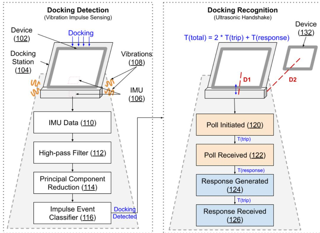
**Fig. 1: Recognizing a docked device via impulse sensing and ultrasonic handshake**
