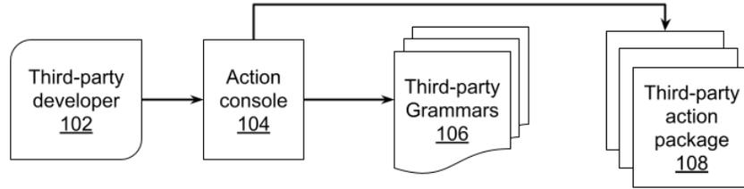
**Fig. 1: Creation of actions (which include grammars and fulfillments) by third-party developers**
