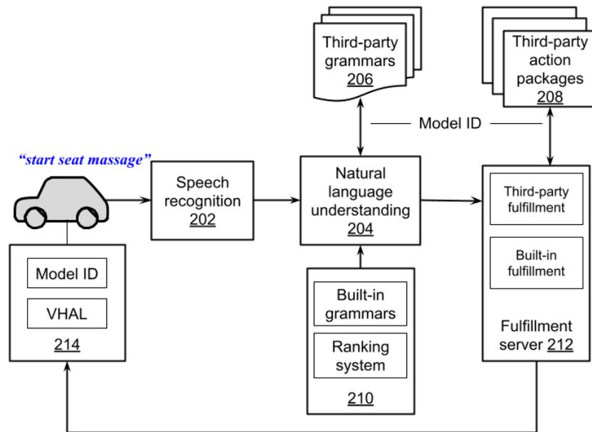
**Fig. 2: Implicit Invocation of Custom Actions in a Vehicle using a Virtual Assistant**
