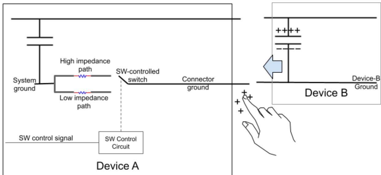
**Fig. 4: Electrical schematic of transient suppression using smart control of the impedance to ground**
