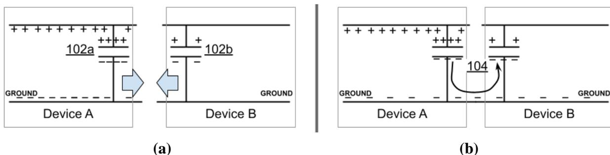
**Fig. 1: Origins of a transient event: (a) Just prior to connecting devices A and B; (b) A strong transient current flows just after the ground connection is established.**
