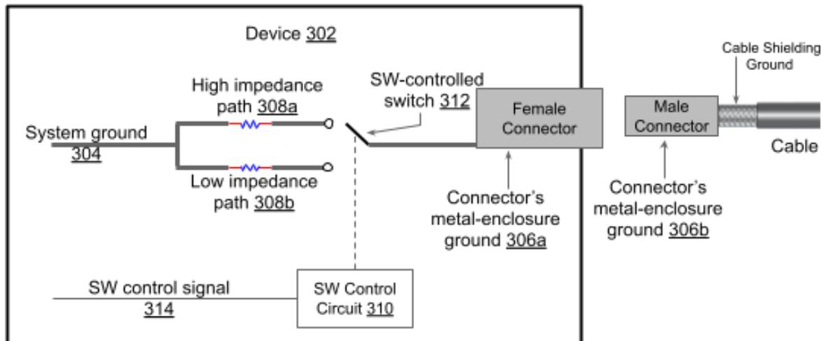
**Fig. 3: Suppressing electrical transients using smart control of the impedance to ground**
