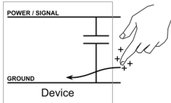
**Fig. 2: Electrostatic discharge giving rise to a transient event**
