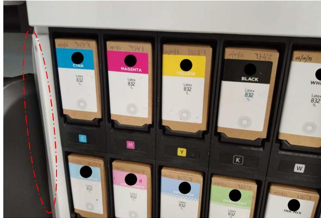
Figure 2. Example of a possible location of the transparent tube for leakage detection
