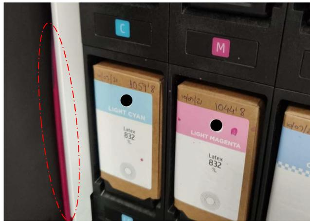
Figure 3. Magenta leakage seen by the customer thanks to the transparent tube
