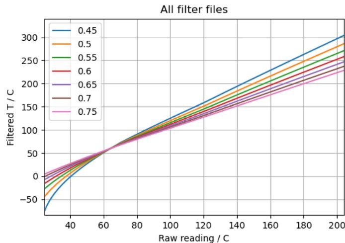
Figure 2: Thermal correction for materials with different emissivities, assuming a reflected temperature of 60C. At the intersection point all the curves the emissivity of the material makes no difference.
