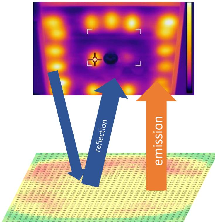
Figure 1: schematic of radiation thermally emitted VS reflected from a surface. Reflected radiation is measured by the thermal camera and contaminates the measurement.
