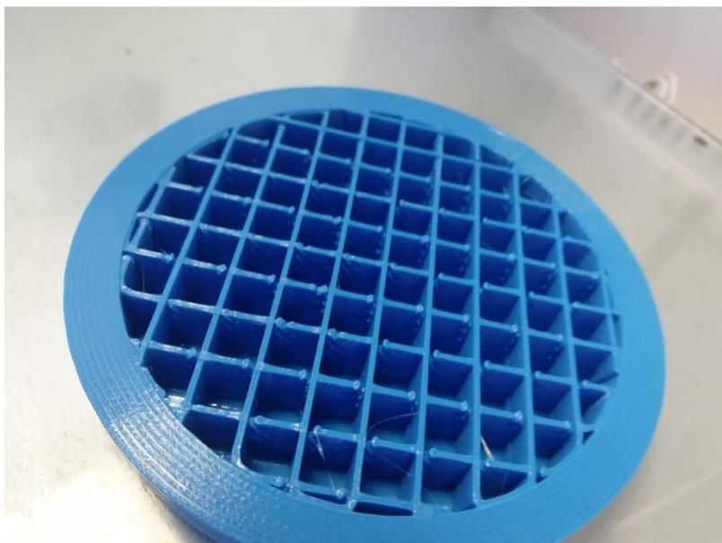
Fig. 1 – Grid infill as printed on Ultimaker printer and AA0.8 nozzle
