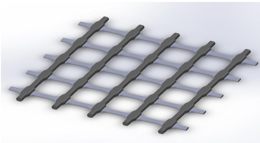
Fig. 4B – Second layer of RELIS. Parameters [mm] – Infill line thickness 0.5\*, Layer Height 0.15\*, Reinforced parts line thickness 0.8, Line spacing 3
