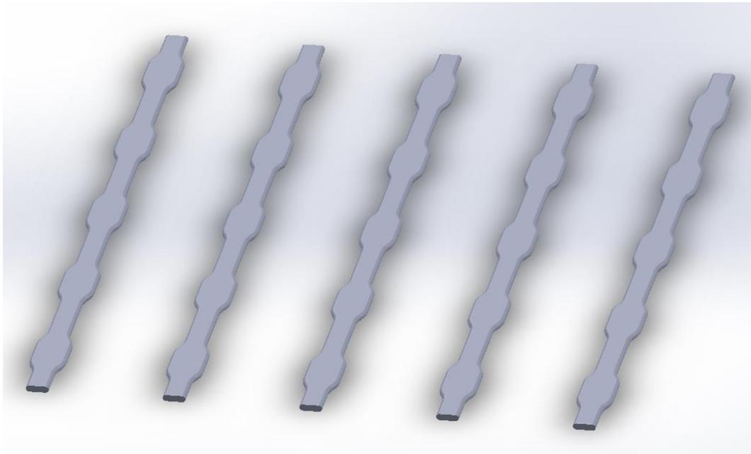
Fig. 4A – First layer of RELIS. Parameters [mm] – Infill line thickness 0.5, Layer Height 0.15, Reinforced parts line thickness 0.8, Line spacing 3
