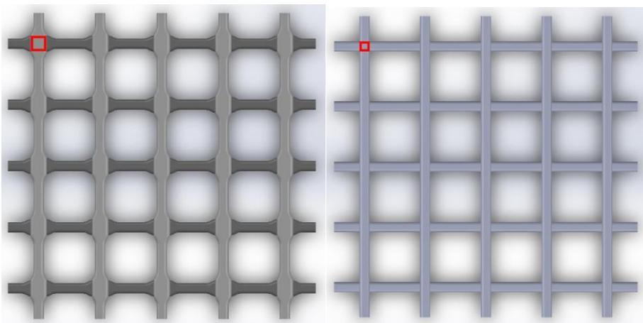
Fig. 7 – Comparison of bonding surfaces in the infill line intersections (RELIS on the left, Line infill on the right)
