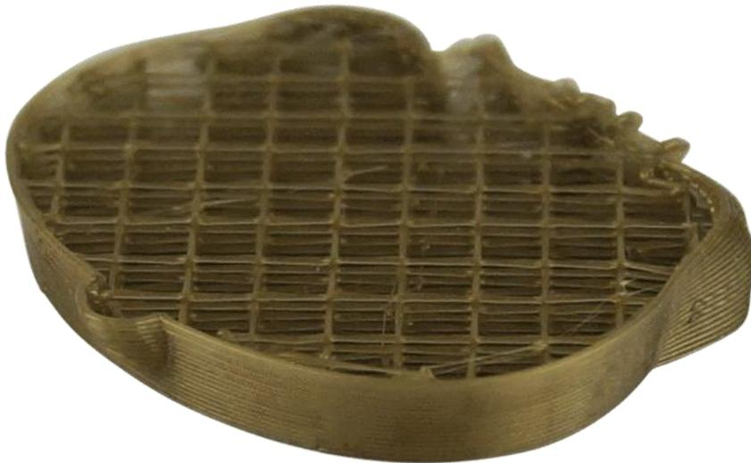
Fig. 2 – Lines infill showing circular extrusion lines not connecting with the previous layer (Figure source: <https://rigid.ink/pages/ultimate-troubleshooting-guide#issue-deformed-infill-22>)
