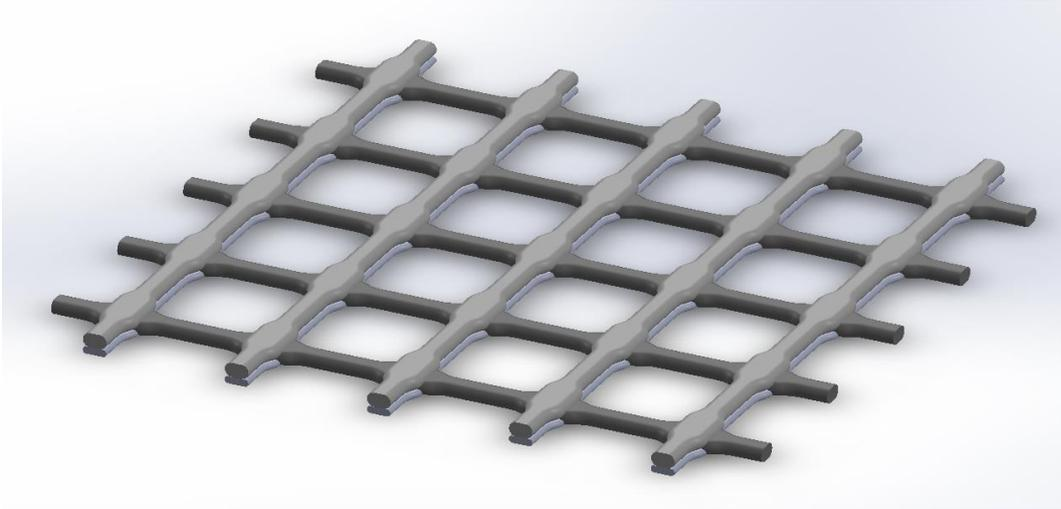
Fig. 5 – Third layer of RELIS. Parameters [mm] – Infill line thickness 0.5\*, Layer Height 0.15\*, Reinforced parts line thickness 0.8, Line spacing 3
