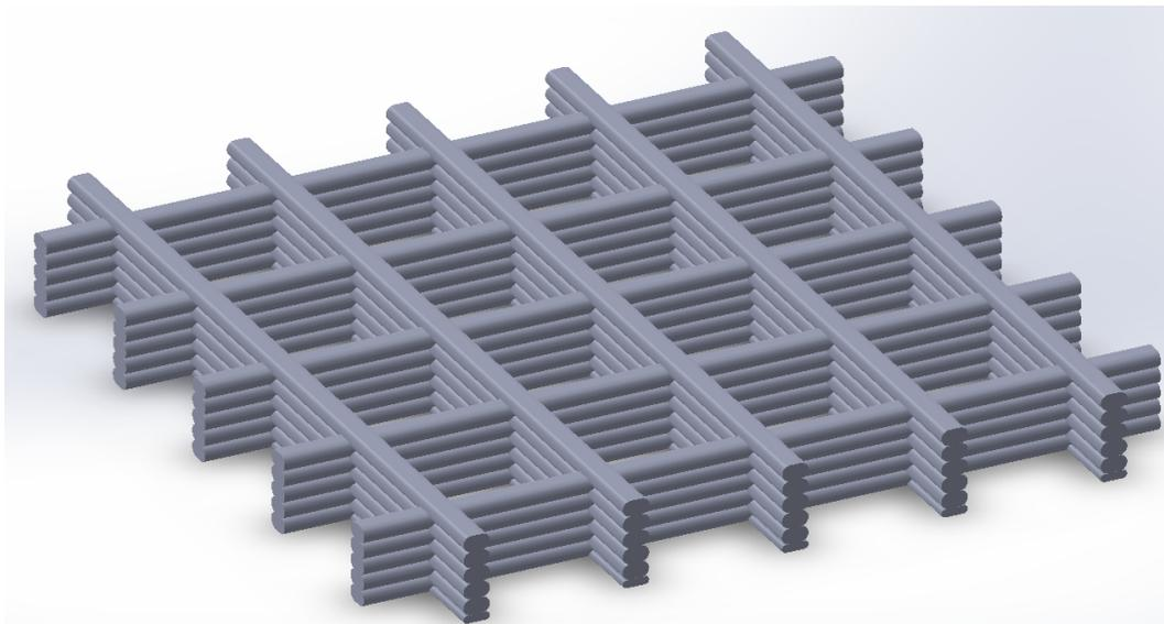
Fig. 3 – Interlocked lines infill structure acc. prior art
