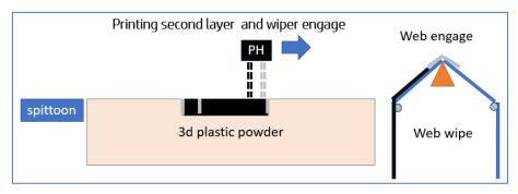
5) Finally the printhead will perform the wiping, with a clean web impregnated with DA
