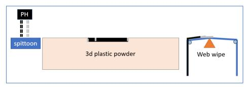
4) Then will travel back to the wiper side, printing one new layer. Before arriving to the wiper it will engage so the printhead and the web has the wiping interference needed.
