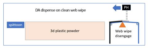
2) After this, printheads travel across the bed printing the content for the layer that will be part of a 3D printed part later on using all agents.
