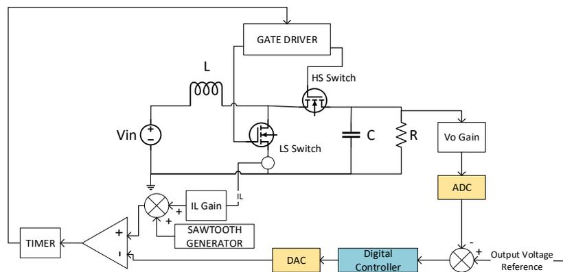
Figure 3. DCDC Boost Converter under Digital PCMC when current sense is implemented on the LS, and slope compensation is applied directly on the sensed inductor current.
