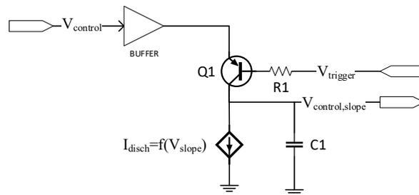
Figure 7. Generic implementation of the proposed slope-compensation circuit.
