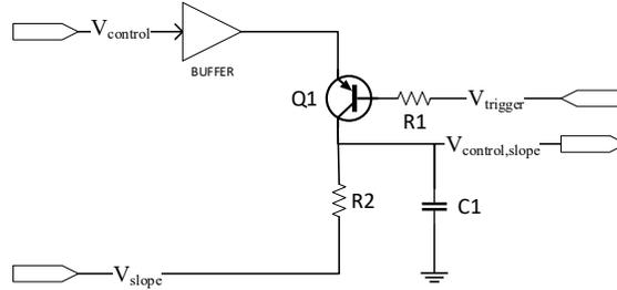
Figure 8. Implementation of the proposed slope-compensation circuit (Approach 1 – Resistive Discharge).
