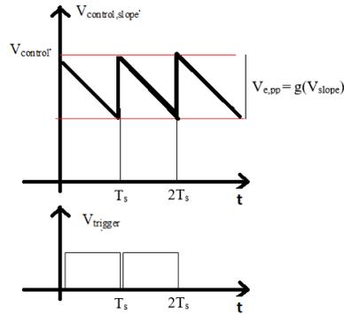
Figure 6. Ideal  $V_{control,slope}$  slope-compensated control signal.
