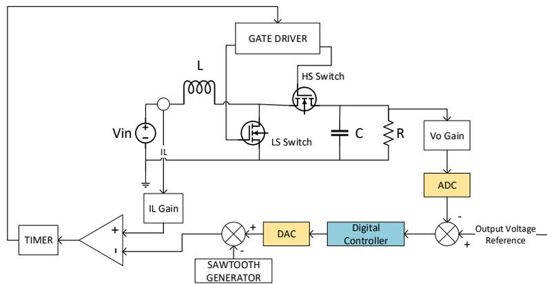
Figure 2. DC-DC Boost Converter under Digital PCMC when current sense is implemented on the HS, and slope compensation is applied on the control signal that sets the targeted peak inductor current.
