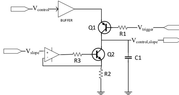
Figure 10. Implementation of the proposed slope-compensation circuit (Approach 3 – NPN BJT Current Source in Negative Feedback Configuration).
