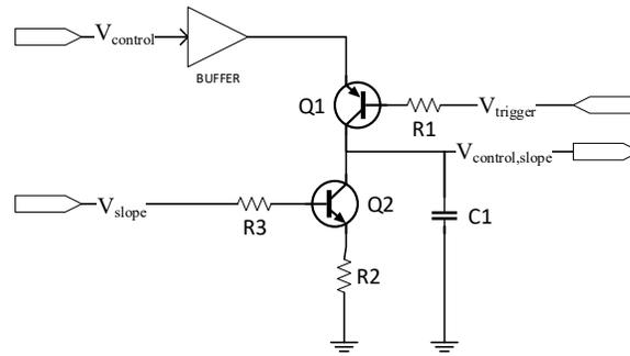
Figure 9. Implementation of the proposed slope-compensation circuit (Approach 2 – NPN BJT Current Source).
