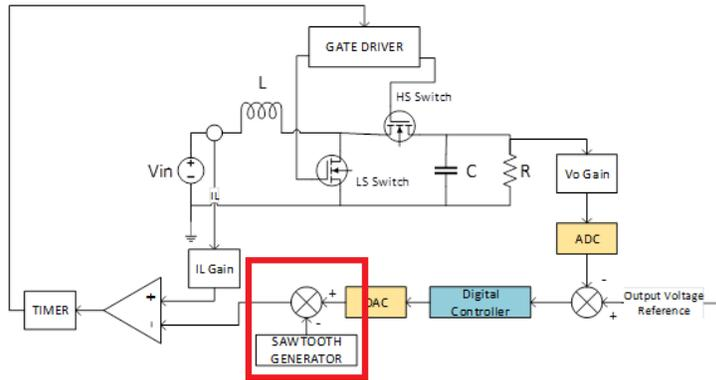
Figure 4. Block implemented by the proposed solution in the digital PCMC scheme.
