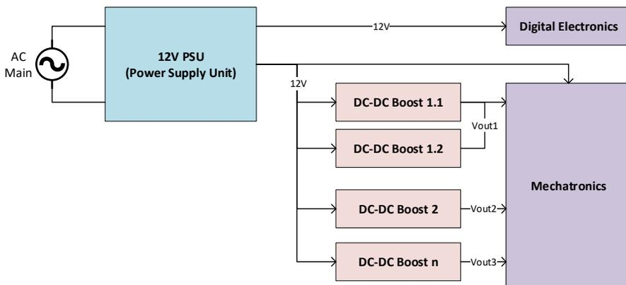
Figure 1. Typical simplified power architecture of Large Format Printing products targeting low cost.
