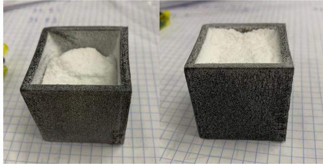
*Figure 2: Prior powder collection closed cubes. Observe that powder inside is more caked than normal.*
