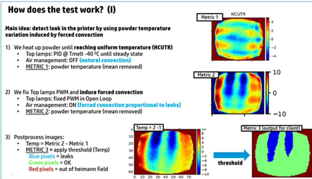
• Figure 1 Main Functional Block of the Air Leak Test
