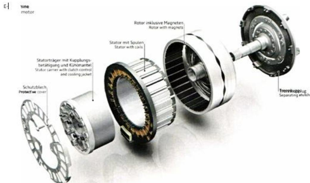
Figure 1: Exploded view of the external rotor e-machine of the Audi Q7 e-tron.
