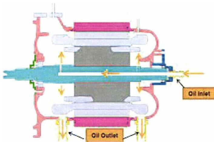
Figure 2: Sectional view of an internal rotor E-machine with direct cooling (source: <https://ieeexplore.ieee.org/document/8507058>)
