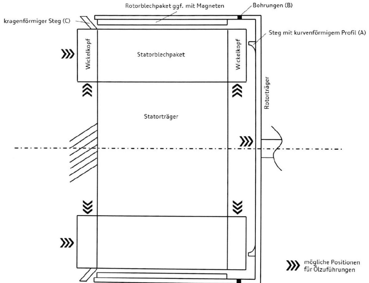
Figure 3: Sketch of a possible implementation as a sectional view.
