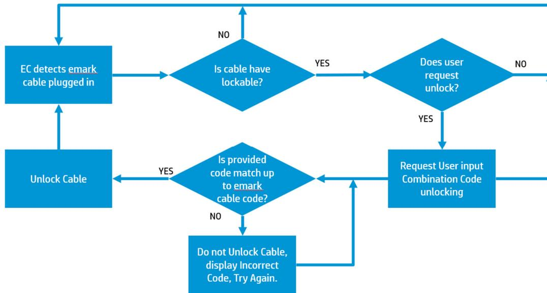
Figure 4: A flow chart showing the steps needed for detecting, locking and unlocking of a lockable USB cable.
