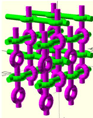
One way to alternate the directions of the loops results in a dense packing with a high number of interlocking loops per volume:
