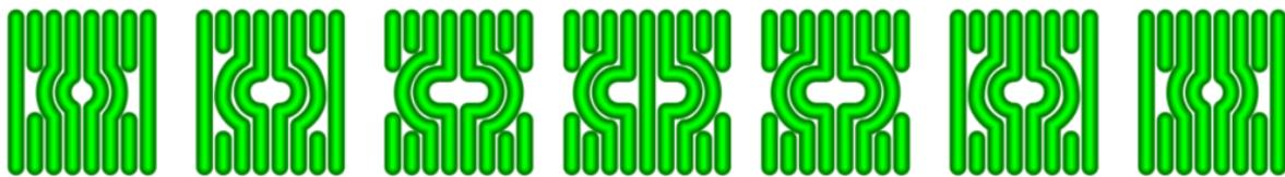
The toolpaths close to the cavity are kept constant, while some toolpaths farther away are cut into pieces.
