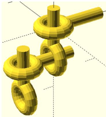
When using this method to improve the adhesion between different materials, one could print these chains in one material, surrounded by toolpaths done in the other material.
