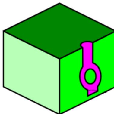
A cavity is created in the first material which cavity is isomorphic to a torus and two cylinders and spans several layers, see below.
