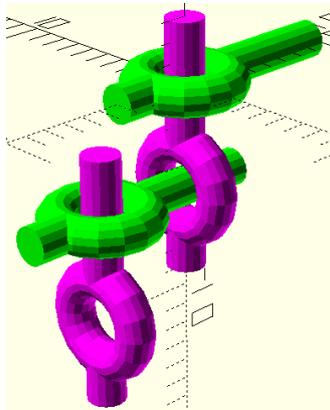
These chains could be laid down in a grid, such that an interlocking structure is formed where every X layers of the first material, the second material is injected downward around and through continuous toolpaths of the second material at a lower height. (In the following the color of the loops does not necessarily refer to the material; instead green signifies horizontal loops and magenta vertical loops.)
