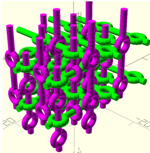
The benefit of the above solution is to increase the adhesion of layers in the Z direction – whether those layers are printed with the same or with a different material. When subjecting a products to tensile forces, the ultimate yield strength will be higher, compared to normal planar layers.
