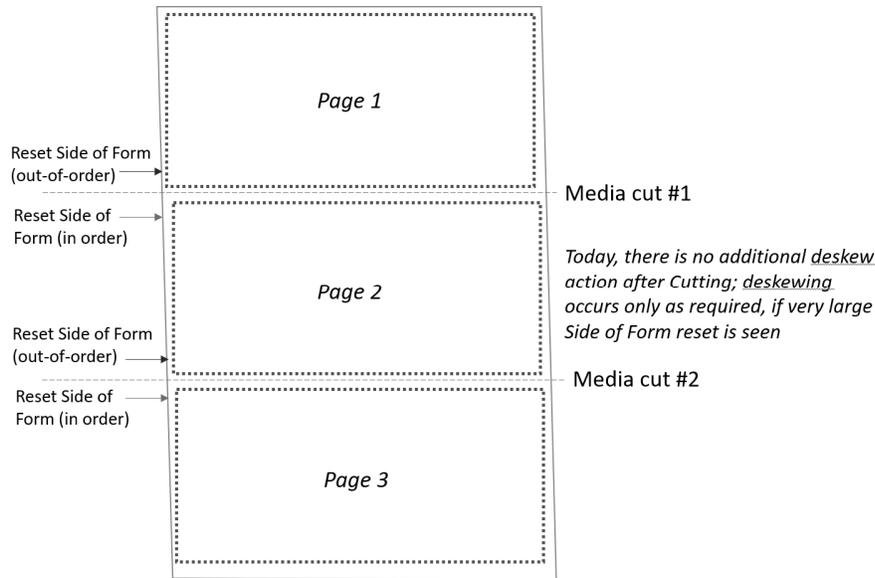
Figure 3: Diagram showing how re-sensing Left Edge on Roll-Media does not need to be in-order
