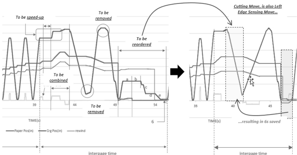
Figure 2: Diagram of Non-Printing actions (focused on Carriage) re-ordered and/or reduced To this end, it was found that, with deeper understanding of roll sheet behavior during the printing and cutting process, it was possible to reorder execution of key non-printing actions. The key learning was, that it was possibly to not just re-order the Left Edge Sensing action to coincide with Cutting (see how this is safe, in Figure 3), but also do it with significant direct and indirect benefits.
