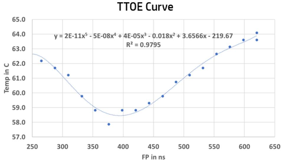
Figure 1: Thermal turn on Energy Curve. The minimum energy for the Fire Pulse to eject is close to 400 nano seconds.
