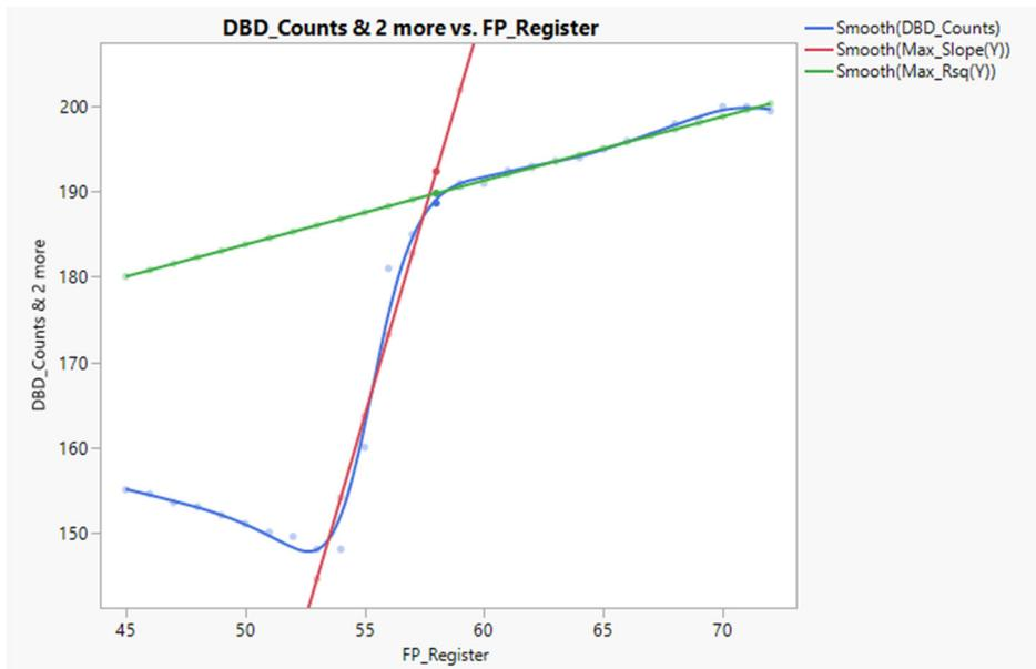
Figure 2: DTOE Curve (blue). The DBD response is plotted vs FP Register setting (Energy). The red line is based off an algorithm to find max slope of 6 data points. The green line is based off an algorithm to find 6 data points higher in energy than the max slope with a high R-squared value.
