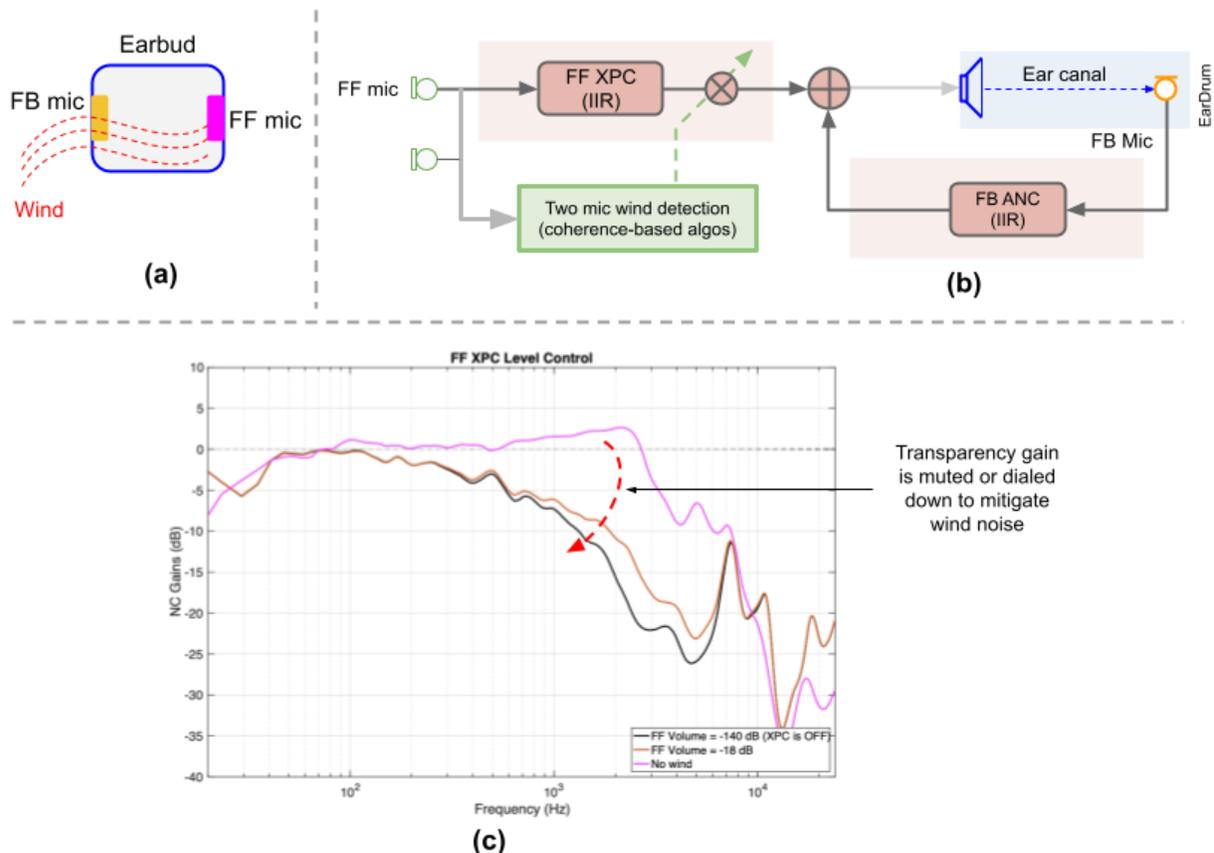
**Fig. 2: Conventional: transparency gain is reduced to mitigate effects of wind noise**
