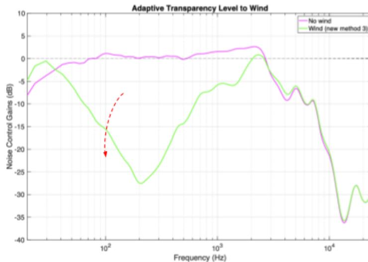
**Fig. 5: Gain of the XPC filter is adjusted based on the detected wind noise**
