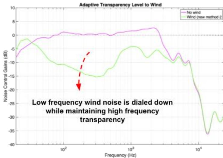
**Fig. 4: Gain of an FIR filter is adjusted based on detected wind noise**
