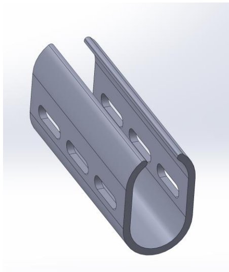
Fig. 7 – Inward-bent radii flexible member
