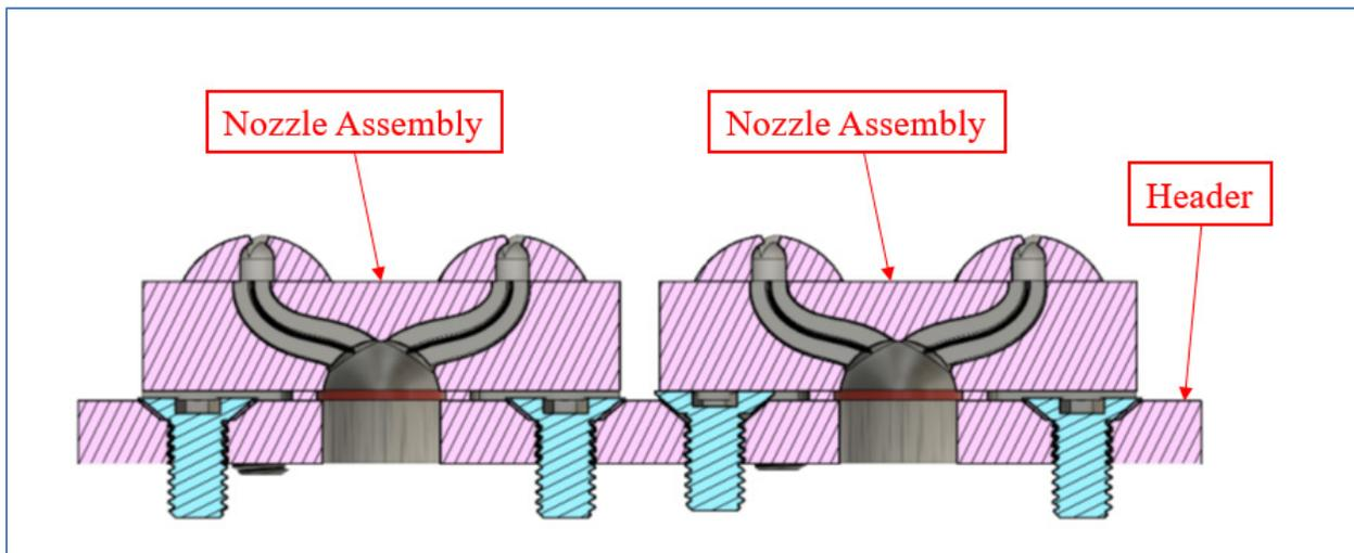
**Fig. 3 – Sectional View of Improved Nozzle Assemblies and Header**
