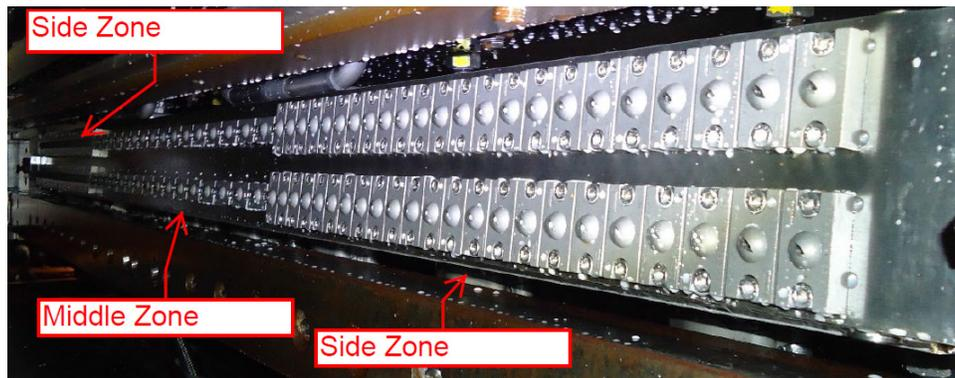
**Fig. 1 – Traditional Cooling Spray Header**
