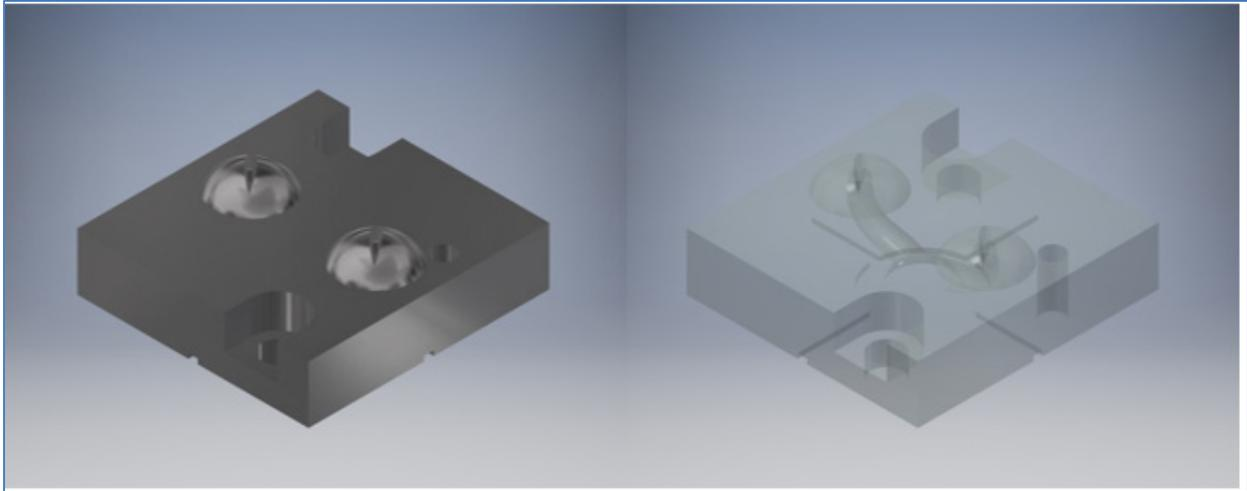
**Fig. 3 – Assembled Nozzle Assembly**
