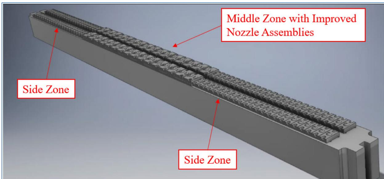
**Fig. 4 – Cooling Spray Header with Middle Zone having Improved Nozzle Assemblies**
