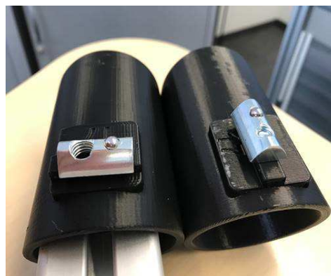
screwable with slot nut for fastening
