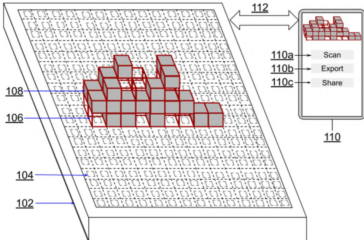
**Fig. 1: A hardware interface and accompanying software to intuitively model voxel-based 3D objects**
