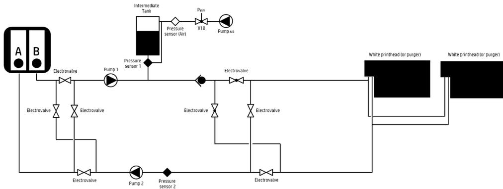
Figure 1. Schematics of an Ink Recirculation Delivery System with an Intermediate
