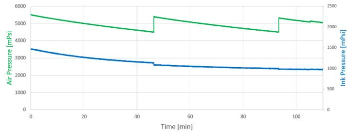
Figure 3. Ink drooling detected based on Pressure drop
