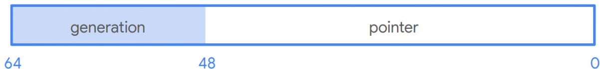
Fig. 2: Using the upper 16 bits of a 64-bit architecture to store the generation field of a CheckedPtr with zero overhead
