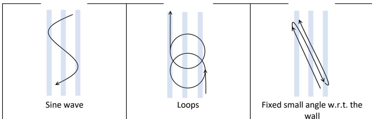
The ironing path strategies shown in Figure 2 are just some examples and it is not an exhaustive list. Other strategies are possible for ironing the wall lines. It is noted that the Sine wave example of Figure 2 resembles the example shown in Figure 1.
