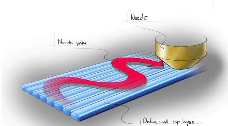
An additional problem to overcome is that if the ironing is being performed perpendicularly to the walls' direction, it will result in a series of short rapid nozzle moves which bring unnecessary vibration to the printer. Advanced travel planner can overcome the vibration issue, but its use would result in slowing down to unusable level.
