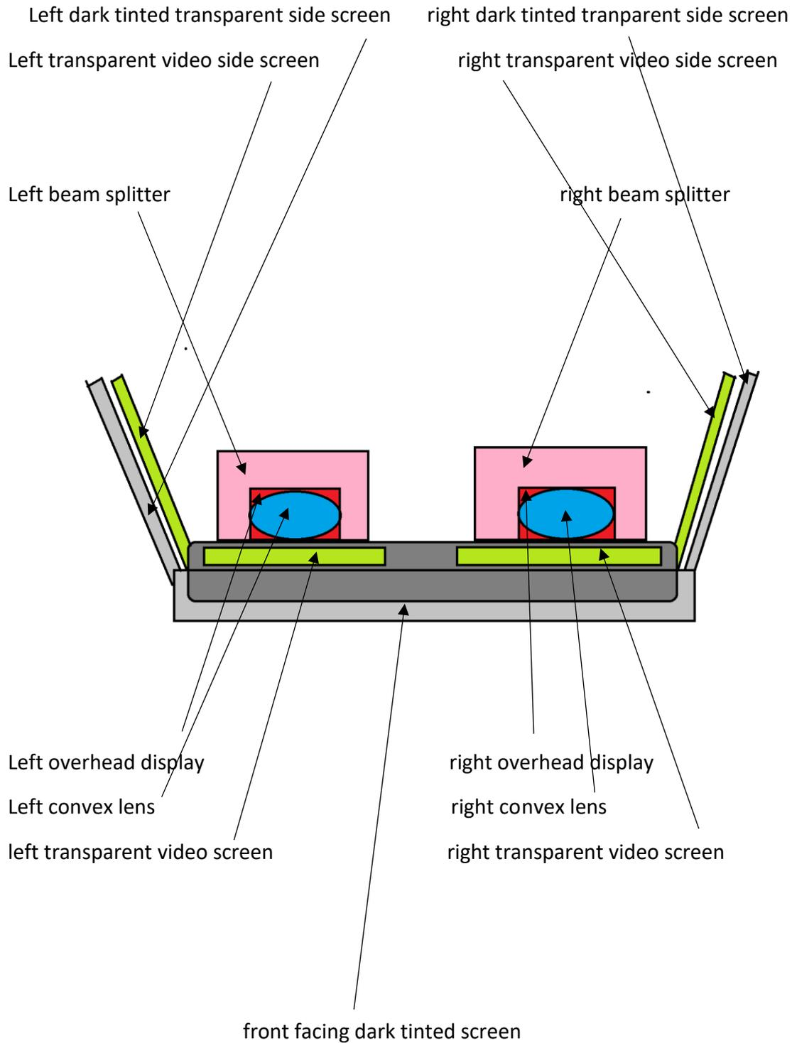
Description of the parts of the head mounted augmented reality display.
