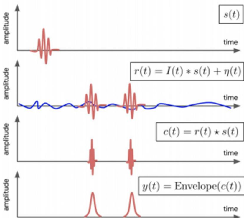
**Fig. 2: Signal processing to detect room temperature**
