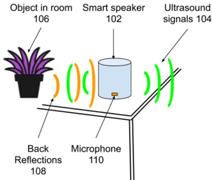
**Fig. 1: Measuring room temperature via ultrasound using a smart speaker**
