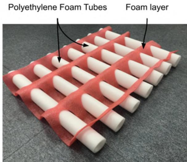
**Fig. 2: View of polyethylene foam based cushion structure**
