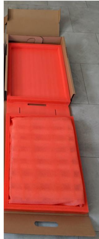
**Fig. 3: Polyethylene foam based cushion used with a packaging box**
