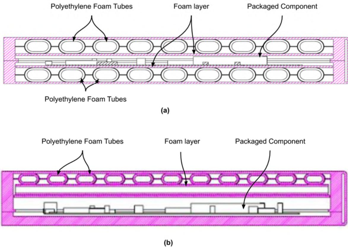
**Fig. 1: Cross-sectional views of polyethylene tube foam based packaging cushion**
