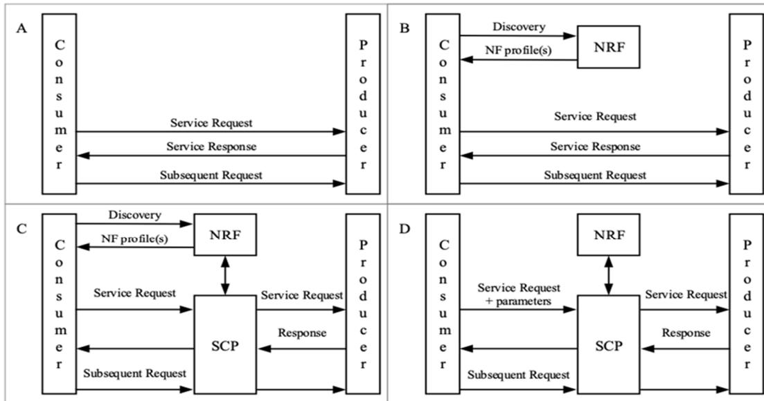
Figure 1: Communication Models for NF/NF Services Interactions
