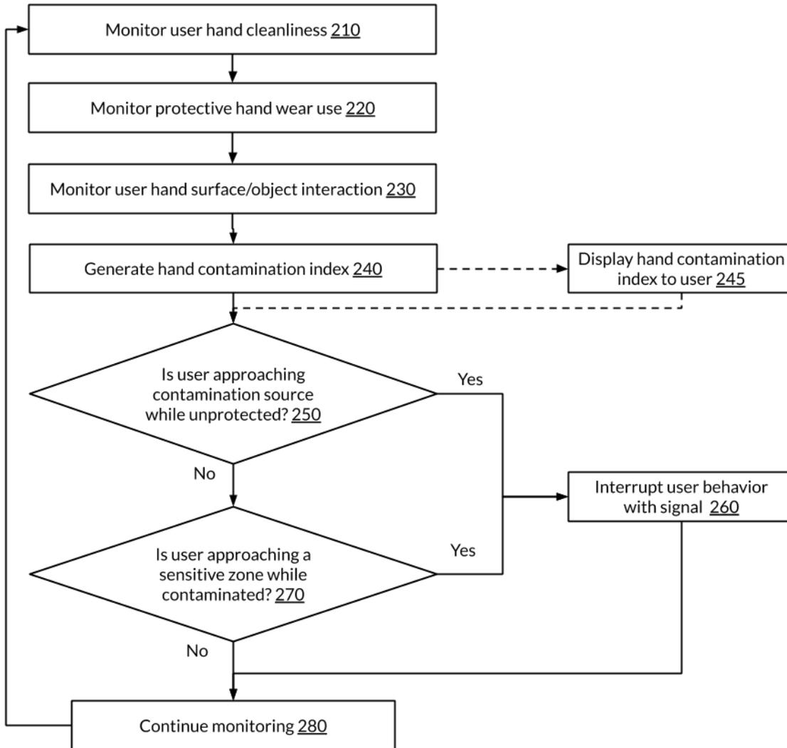
**Fig. 2: Monitoring of hand health and generation of alerts**
