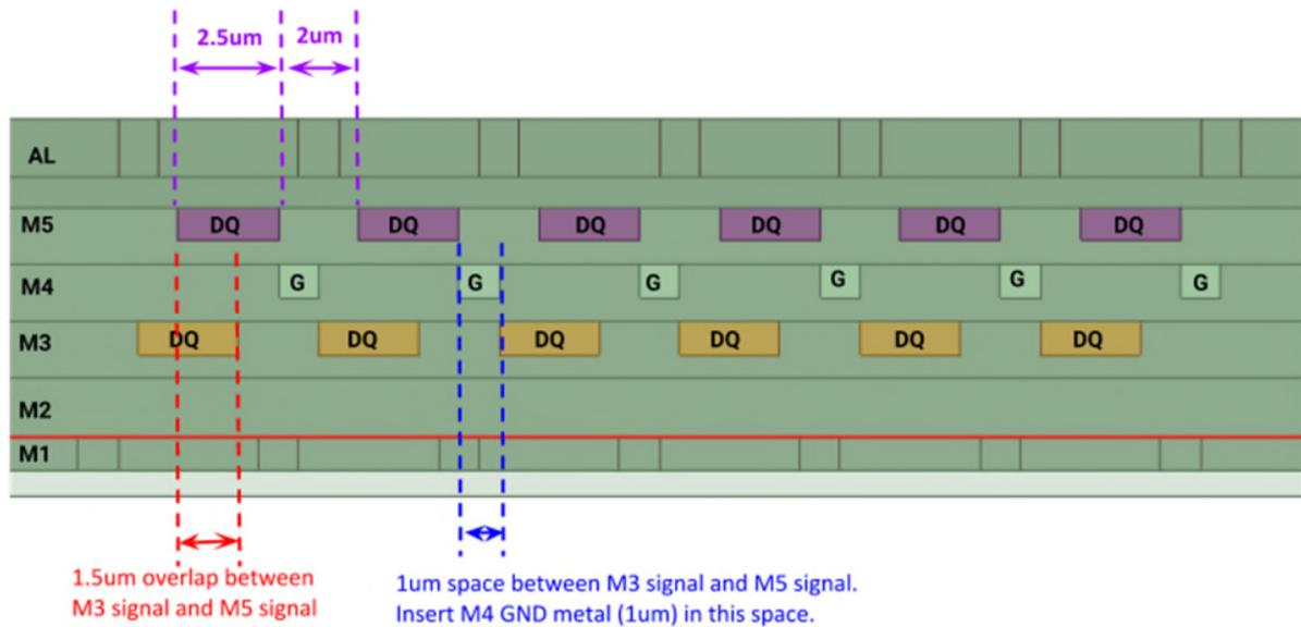
**Fig. 2: Cross-section of a five-metal layered, low-loss, low-crosstalk silicon interposer channel that is robust to inter-symbol interference**
