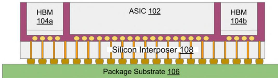
**Fig. 1: An interposer used for data communications**
