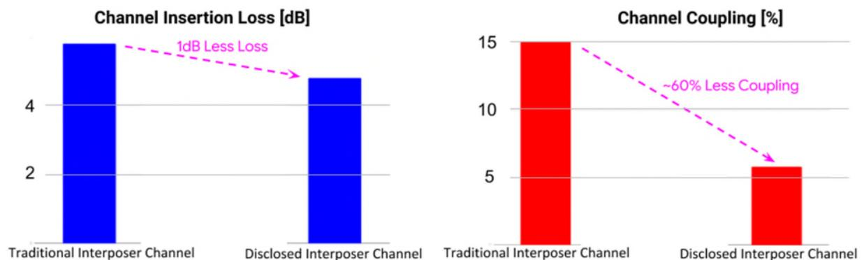
**Fig. 3: Illustration of lower loss and channel coupling**
