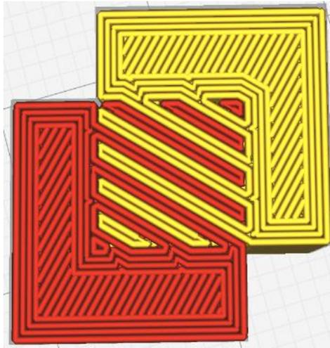
This weaving of beams causes vertical beams to be formed at the intersections of the same material with the different directions. Such vertical beams can be detected in the picture below which only shows one of the two materials. In this picture the regular changing of orientation of the (yellow) fingers is visible. Also, a brim around the object is shown, which is not subject to the invention.
