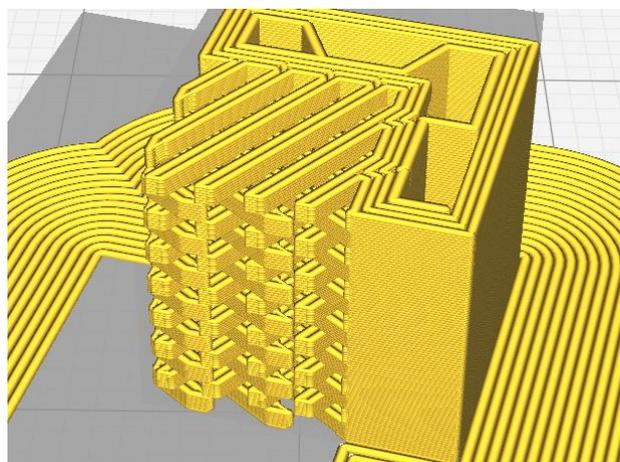
By letting fingers of one material extend into the other material, and by changing the direction of the fingers every X layers, the two materials are firmly locked in all 3 dimensions.
