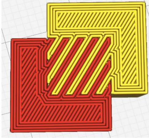
The direction of these beams/fingers is rotated every  $X$  layers, with  $X$  being a preferred number of layers. The rotation angle  $A$  can be chosen such that the pattern has rotated a full 180 degrees (to align with the original direction) in  $N$  rotations, where  $N$  is typically 2 and  $A$  is typically 90 degrees.
